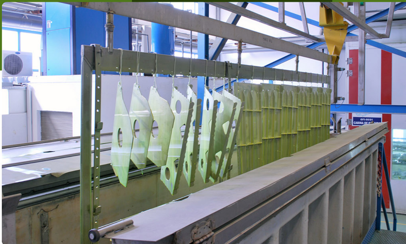
Liquid Penetrant Inspection
