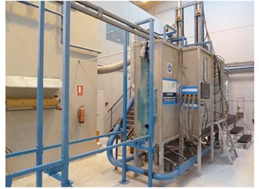
Automatic Glass Shot Peening
